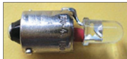
Figure 15 — LED built into base of dial light bulb.
