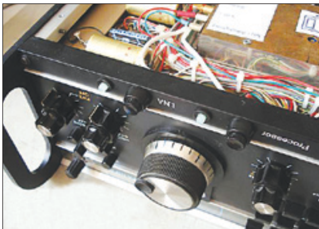
Figure 11 — Installed front panel extension, as seen from the bottom.
