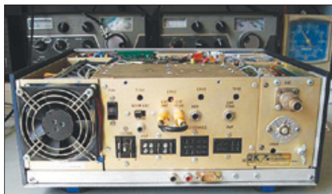
Figure 12 — TR-7 with rear extension installed.
