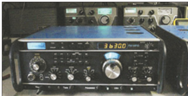
Figure 10 — The new LED display is shown installed in the TR-7.
